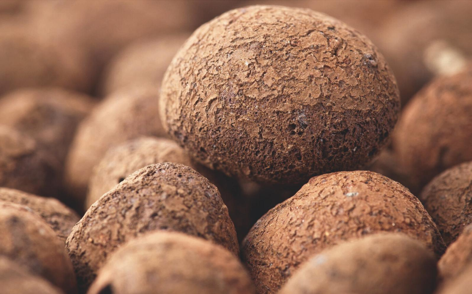
*Expanded clay is a lightweight aggregate that is produced from natural clay. It is suitable for a wide range of applications in the construction sector, such as housing and infrastructure. It can be used in green applications such as in hydro-culture and technological applications (water treatments, roofgardens).*
