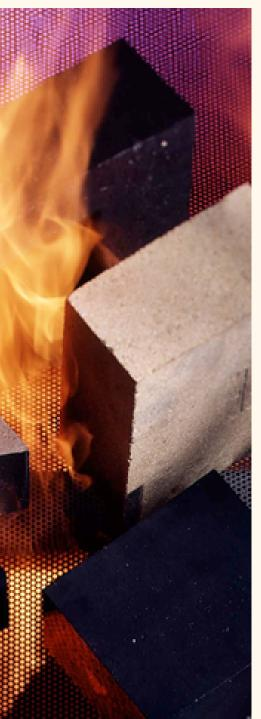
In the refractory industry, manufacturers can produce monolithic refractories and refractory bricks that contain between 20% and 80% of recycled material. Virgin refractory materials can be substituted by recycled material coming from various industries (e.g iron, steel, metallurgical industries, alumina, ceramic, cement). Materials are then sorted, crushed, dried and possibly milled. These products are tailored to the installation method as well as the application conditions of customers.
