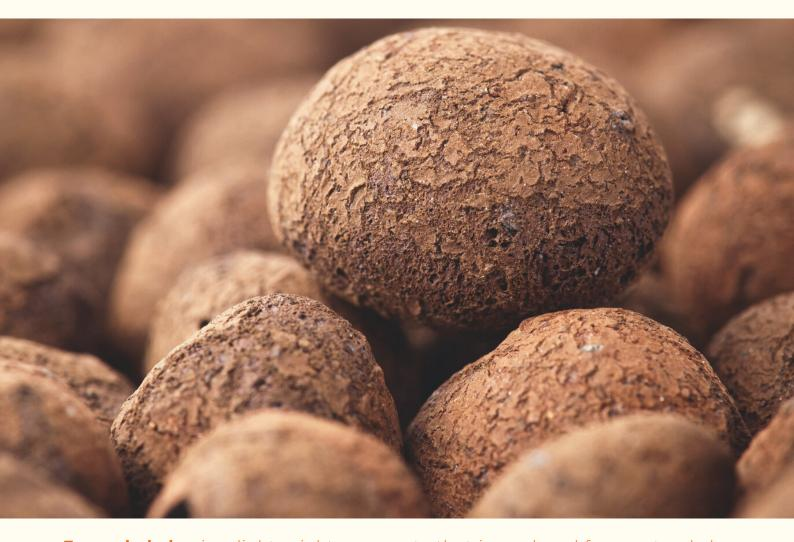
**Expanded clay** is a lightweight aggregate that is produced from natural clay. It is suitable for a wide range of applications in the construction sector, such as housing and infrastructure. It can be used in green applications such as in hydro-culture and technological applications (water treatments, roofgardens).
